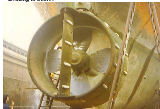
Four bladed pitch controlled stainless steel propeller with Kort-Nozzle
